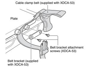
**2** Bundle the three connection cables with the cable clamp belt. Pass the cables as illustrated.
